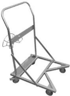
The trolley makes it easy to move the equipment between different working places. The trolley's base plate has the same height as a standard pallet and a V-shaped front which positions a big part of the drum over the pallet before it leaves the trolley. A very stable construction that delivers a reliable usage.
